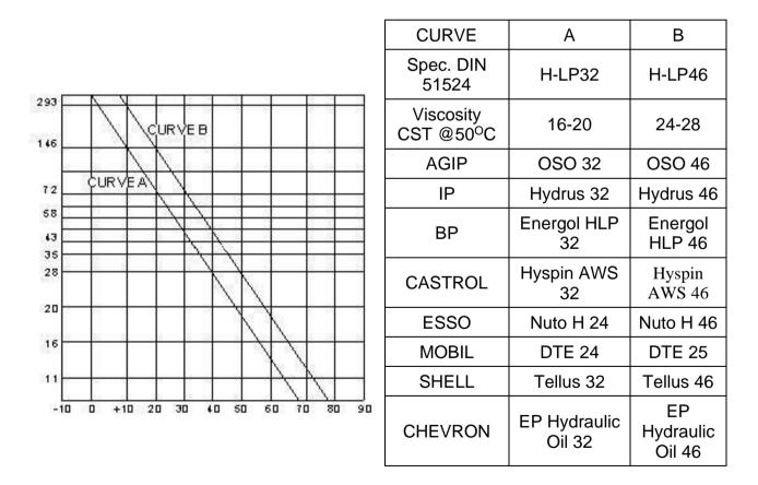
Taking into account that the optimal use conditions for the system are those in which the oil viscosity is around 28 CST in operating conditions, from the reported tables it is possible to determine the most suitable oil category and to choose between the proposed brands (not binding).
