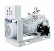
Engine-compressor set driven directly by electric motor flanged to the compressor. Equipped with a control system and can be equipped with a regulation system to work over long periods at a constant operating pressure. This is the best solution for a permanent installation with electric outlet at the offload point.
