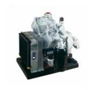
Engine-compressor set, directly driven by hydraulic motor, forming a robust and compact set. Equipped with a cooler to cool the oil in the hydraulic circuit and with a fan driven by the compressor crankshaft.
