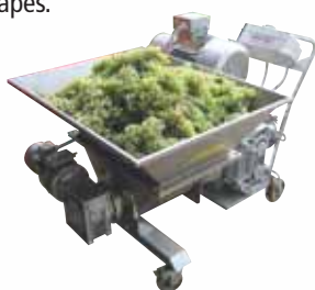
Rotary lobes pump type PL 4000 for pumping of whole grape
