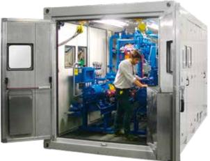
In particular, as regards the supply to gas engines, a gas flow variable in time is required. The rotary vane compressor is a positive-displacement machine and therefore its flow rate, at fixed speed of rotation, is nearly constant.
