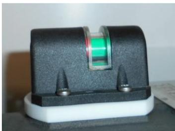
Filter restriction indicator (in the green OK) fully red then filter needs cleaning .
