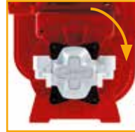
Version H MEC 2000: Group 3 26.7 cc/rev - Pmax 280 bar - In G 1" - Out G 3/4" MEC 3000: Group 3 26.7 cc/rev - Pmax 280 bar - In G 1" - Out G 3/4" MEC 4000: Group 3.5 43.98 cc/rev - Pmax 250 bar - In G 1" - Out G 1"
