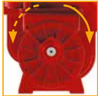
Version P Smooth Cylindrical shaft Ø 22, lenght 48 mm Parallel key UNI 6604
