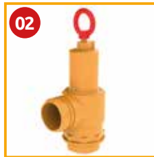
02 Overpressure Safety Valve - 1 1/4 Code 5100200009 Setting range: +0,3 bar / +1,5 bar Working temperature: -20°C / +90°C Thread: G 1 1/4 Weight: 0,94 kg
