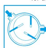
Rotary vane vacuum pumps, oil recirculating type and oil free
