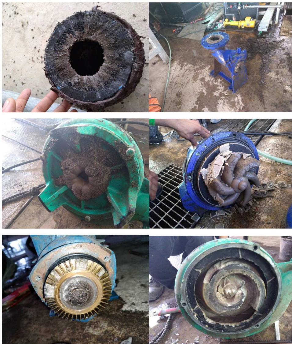
Damage to circulation pumps caused by phosphorus-based crystal deposits (Uslar et al., 2019b).
