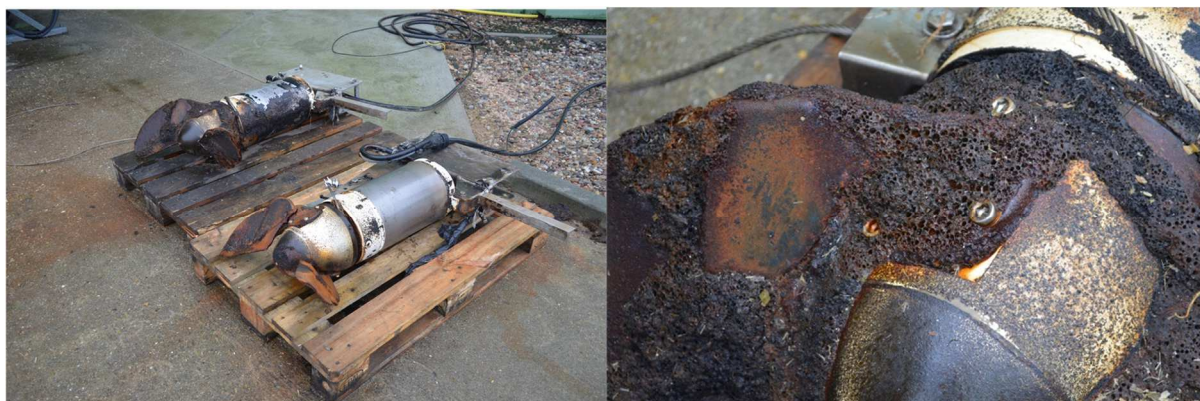
Examples of immersed mixers damaged by wear and crystalline deposit.
